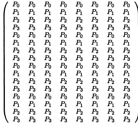
FIG. 7. Wrap mapping of 16 rows to four processors.
